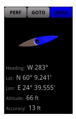
GPS data view (**DATA**, see above) shows a compass arrow which points to the geographic North, heading in degrees, latitude, longitude, altitude above mean sea level and location accuracy.
