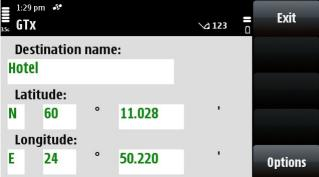
The current location can be set as a destination by touching the navigation circle when GPS navigation data is available. The destination latitude and longitude can also be typed in and the destination name can be edited, see above. Press the # key to get a decimal point. Latitudes and longitudes are in GPS format. Use a conversion calculator (e.g.
